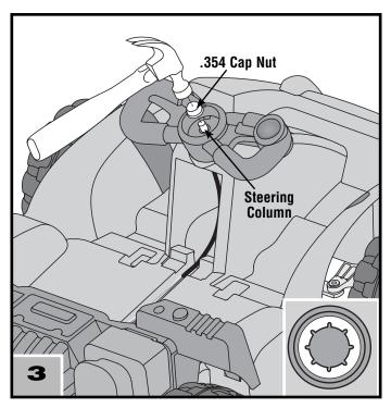
• Fit a .354 cap nut onto the end of the steering column. Tap the cap nut with a hammer to secure it to the steering column.
